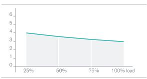
Class-leading THDi of <3% virtually eliminates harmonic distortion of the mains supply.
